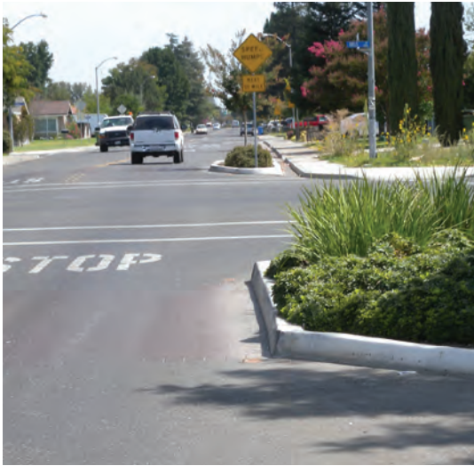
Traffic calming tools, such as curb extensions or intersection 'bulb-outs,' may be used to slow car traffic through neighborhoods.
